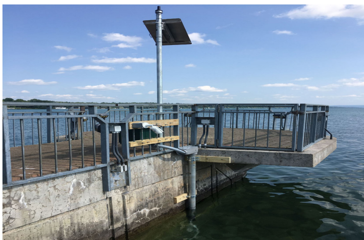
USGS water quality monitoring sensor located on the pier in the Village of Skaneateles, photo credit: USGS
