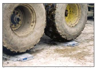
Figure 1: With portable scales, weigh each axle separately.
