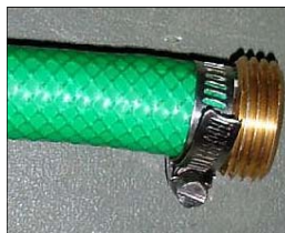
The cut end of the connective hose should be fitted with the male coupling.
